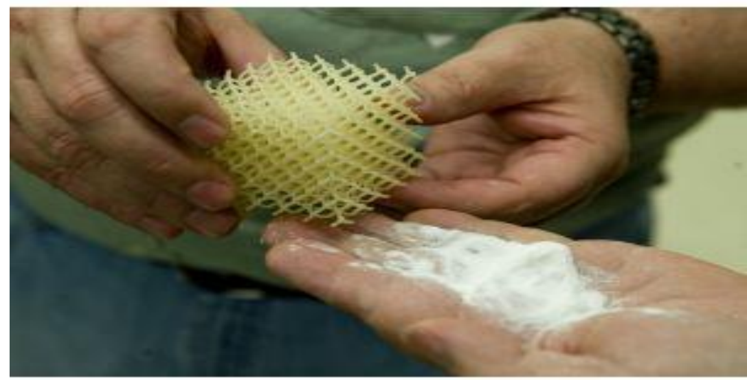
Fig 1: redundant material removal
